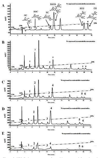
Figure 2. HPLC chromatograms of catechins extracted from the twig extracts: (A) catechin standards, (B) WE, (C) 10% EE, (D) 50% EE, and (E) 95% EE. Chemical structures of catechins: (1) GC, (2) EGC, (3) EC, (4) EGCG, (5) ECG, and (6) CG.
